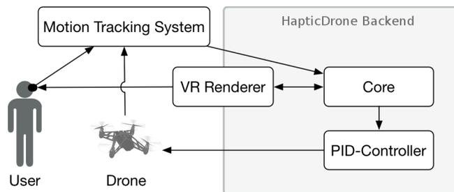
Figure 4. All components of the VRHapticDrones system.
